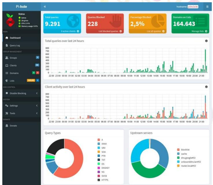
**Pi-Hole: Ad-Blocking System Using Raspberry Pi Fundamentals of Pi-Hole in Network-Wide Ad Blocking**
