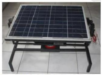
Figure 3: Mechanical Design for solar Tracking
