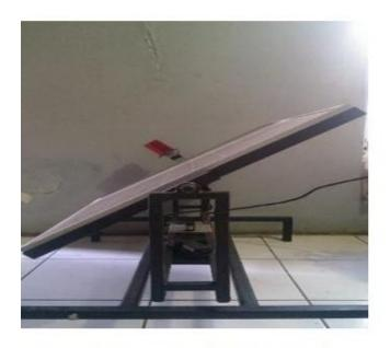
Figure 8: Position of solar panel with -30°C from standard elevation
