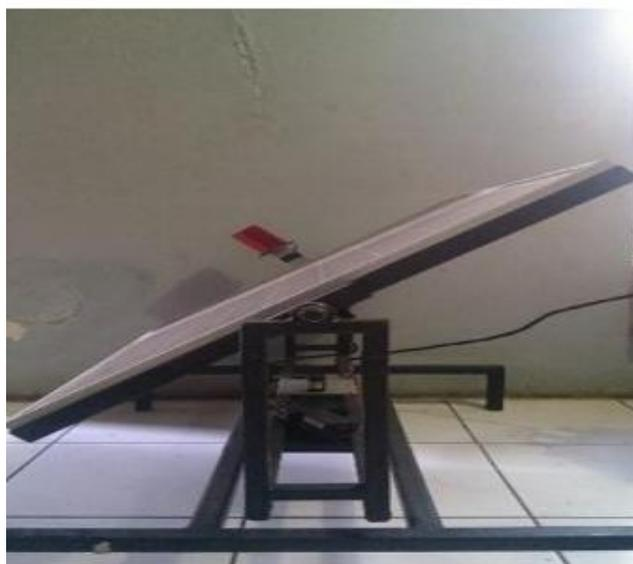
Figure 8: Position of solar panel with  $-30^{\circ}\text{C}$  from standard elevation
