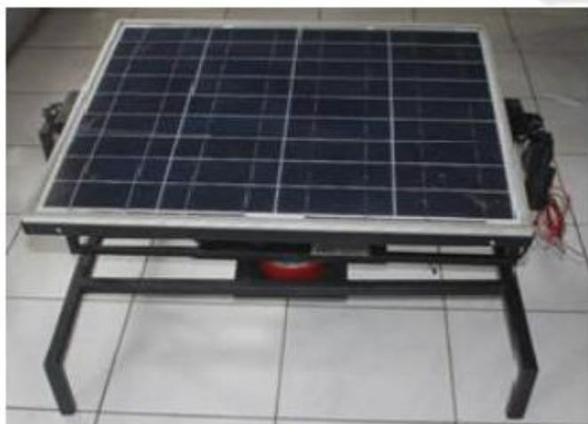
Figure 3: Mechanical Design for solar Tracking
