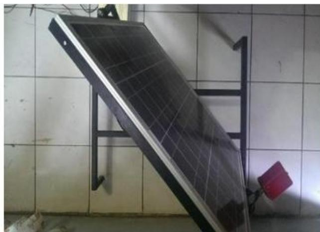
Figure 10: Position of solar panel with -30° from standard rotation
