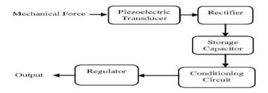
**Piezoelectric Effect:** The project is based on the piezoelectric effect, where certain materials generate an electric charge when subjected to mechanical stress, vibration, or pressure.
