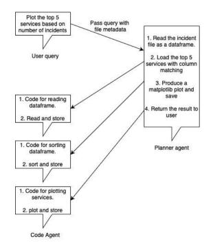
Fig. 6. Generating plan for the sample incident file
