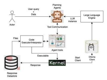
Fig. 1. Architecture of the Proposed System
