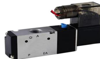
A solenoid valve is a valve that is operated by electrochemically. An electric current is used to control the valve through a solenoid. The solenoid and valve are the two main components of a solenoid valve. The solenoid convert electrical energy into mechanical energy, which is then used to open or close the valve mechanically.
