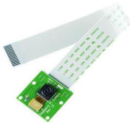
This Raspberry Pi Camera Module Board is a high-resolution 5 MP camera that can take high quality pictures. It does not only take pictures but also shoot videos, making it suitable for drones, CCTV, and other Raspberry Pi projects. A fixed lens with a resolution of 5 MP is built into the camera board. This camera board has a resolution of 2592\*1944 pixels and can capture photographs.
