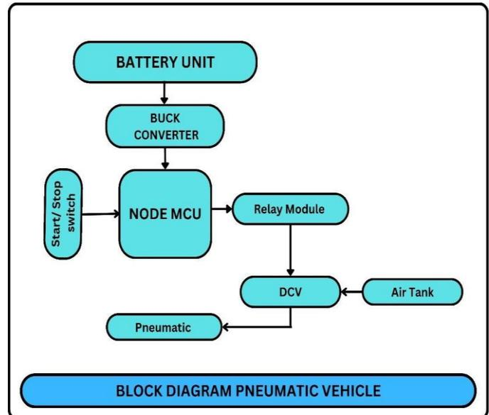
Fig. 1 Block diagram of Pneumatic Vehicle
