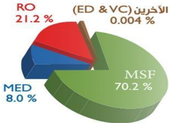
Figure (7): Desalination processes used in GCC countries' percentage contribution (2012)
