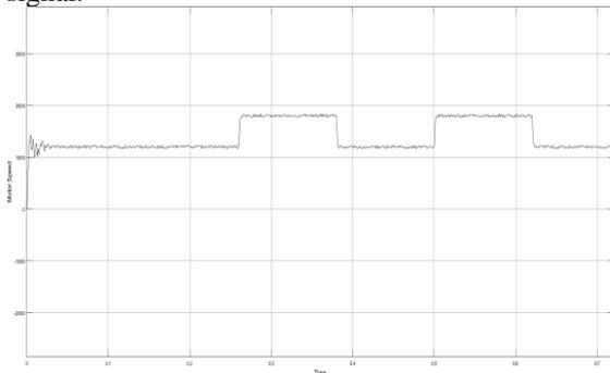
Fig. 10. The controlled motor speed with the transmitted 8-bit signal '11110000'.
