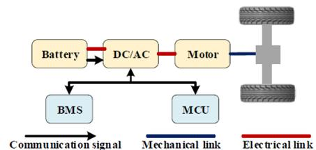
Figure 2: System architecture for an EV employing the P&SMT approach
