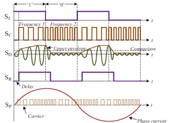
Figure 4: The proposed system's proposed signal transmission scheme,
