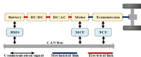
Fig 1: Schematic Diagram of EV integration
