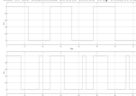
Fig. 8. So represents for the original 8-bit data string and Ss refers to the entire 12-bit transmitted signal.
