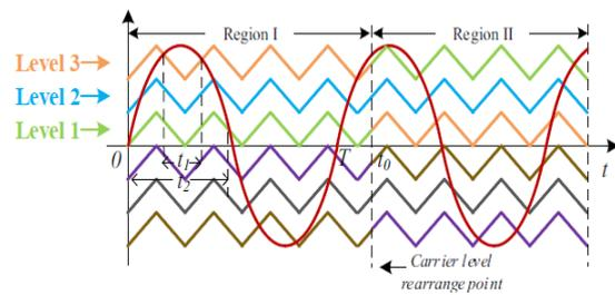
Fig. 5. Carrier level rearrangement in the PWM process.
