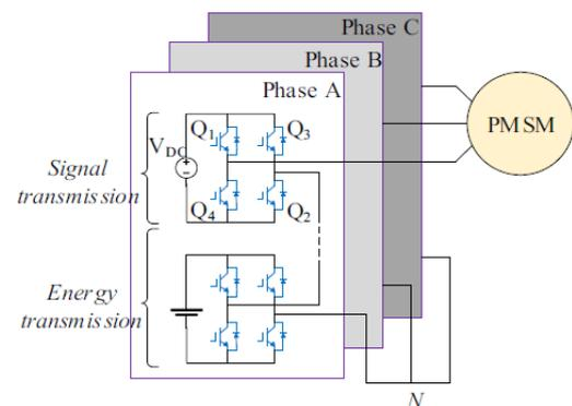
Figure 3. Topology of the proposed P&SMT system for EVs.
