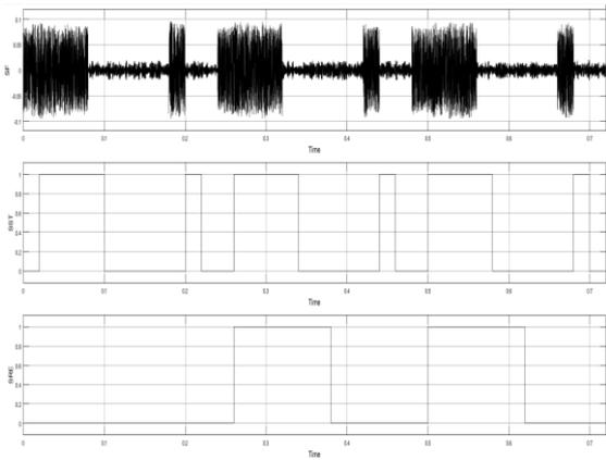
Fig 9 SF represents the extracted 4 kHz carrier after the filtering process; SST is the recovered 12-bit signal; SRE is the restored 8-bit motor speed adjustment signal.
