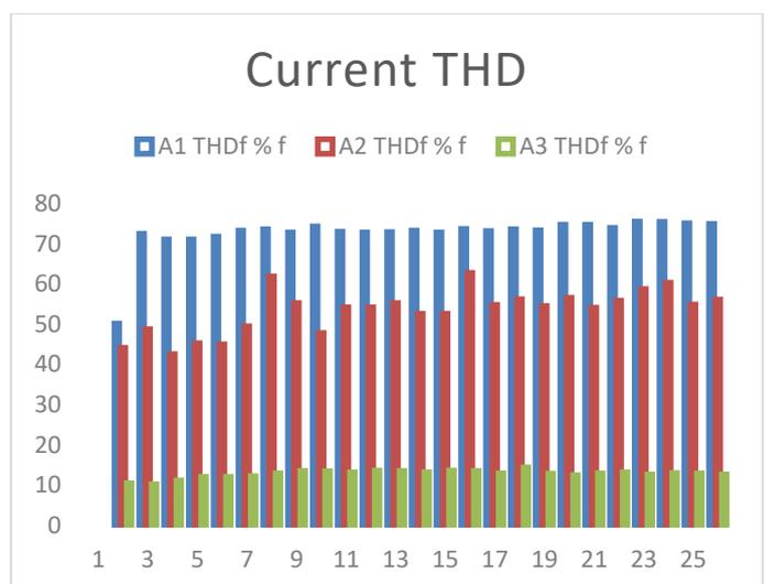
Fig -7: Current harmonics HT side
