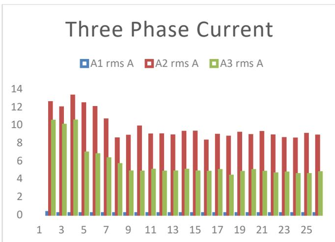
Fig -3: Current harmonics of three phase HT side
