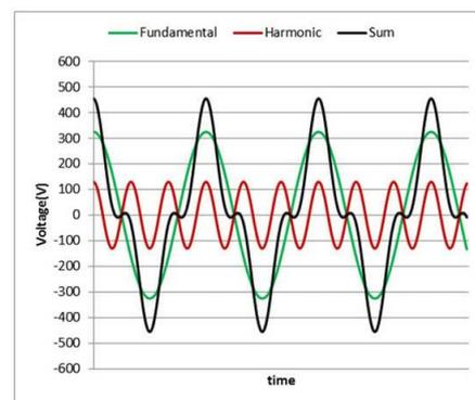
Fig -1: Effect of harmonics in the waveform
