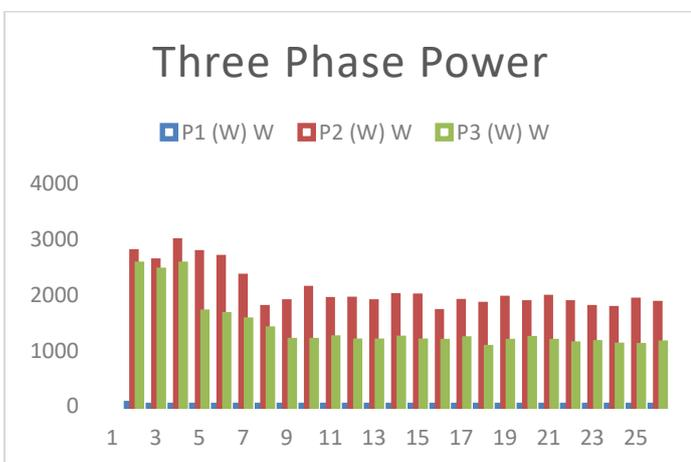
Fig -4: Three Phase Active power
