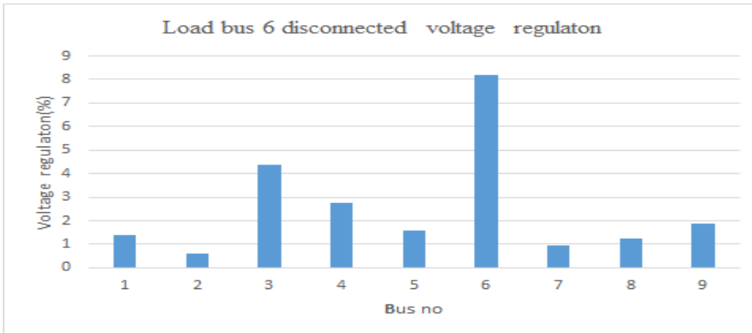
Fig.3 Voltage regulation when load bus 6 disconnected
