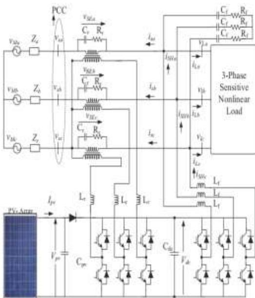
Fig.2.1.(A)System Configuration of Solar Photovoltaic Integrated Unified Active Power Filter
