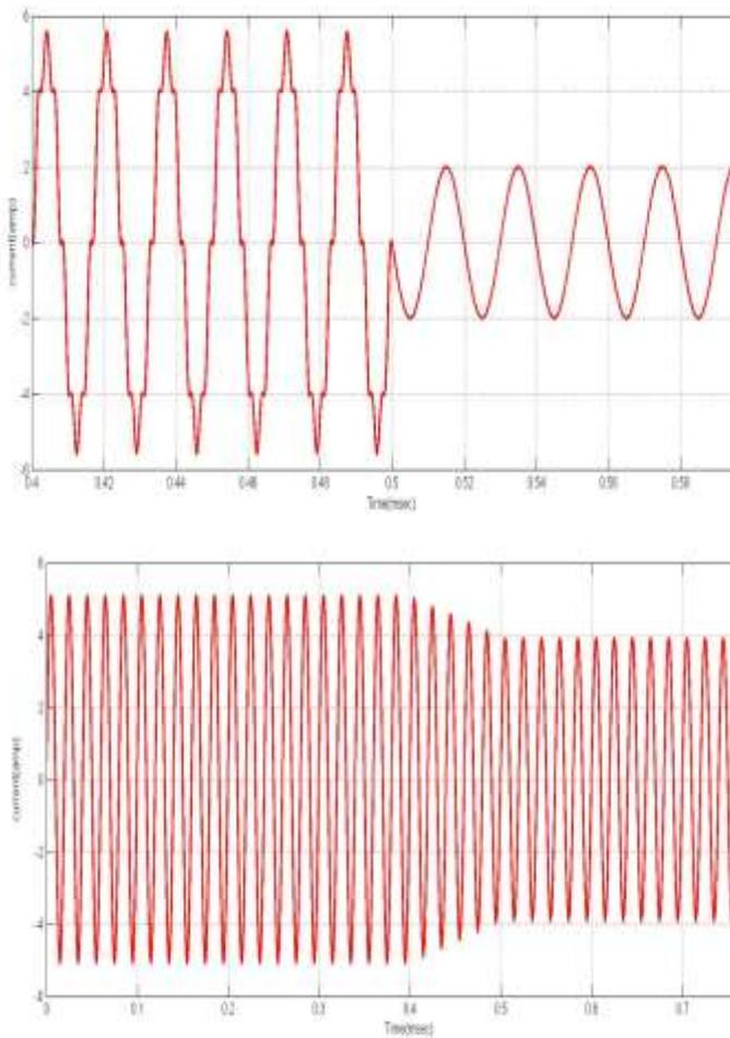
Fig. 3.4(c) Salient Signals in Extraction of Fundamental Positive Sequence Load Current using Adaptive Filter PI controller
