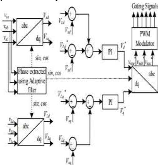
Fig.2.2(B) Control Configuration of Series Active Filter
