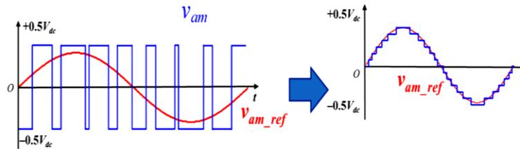
Figure: 3. Waveform in the two-level voltage source and Modular Multilevel Converter
