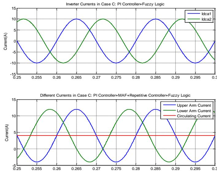
**Figure: 9.3. Simulation Waveforms of Case C: PI Controller, Moving Average Filter followed by Repetitive Controller with Proposed Fuzzy Logic Controller.**
