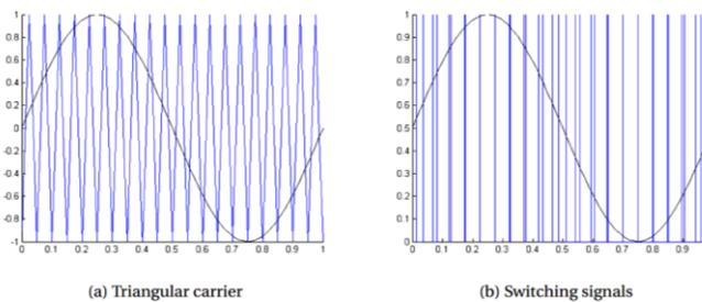
Figure: 6. Principle of PWM switching scheme.
