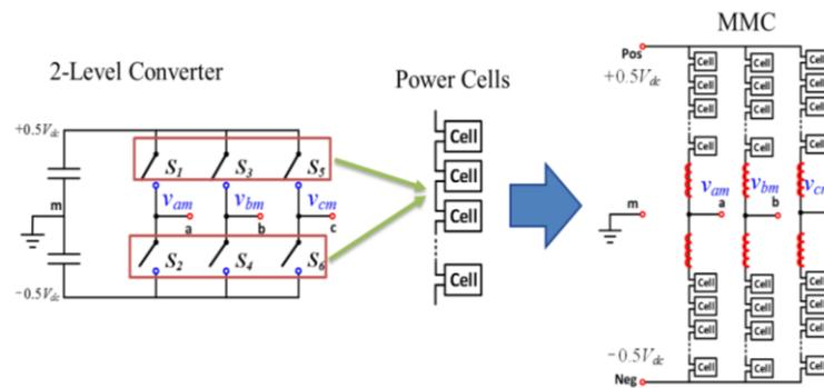
Figure: 1. Modular Multilevel Converter conceptual realizations
