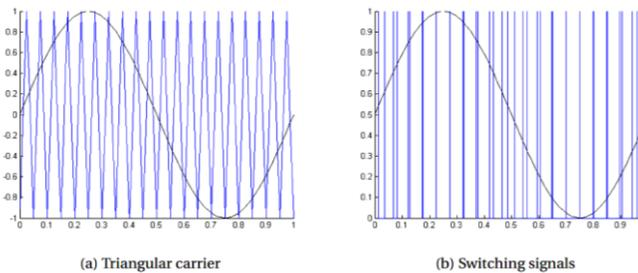
Figure: 6. Principle of PWM switching scheme.
