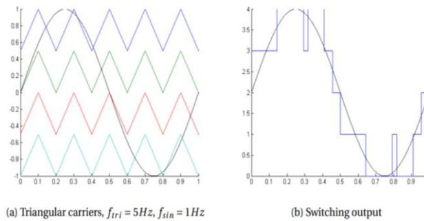
Figure: 7. Level-shifted PWM switching scheme.
