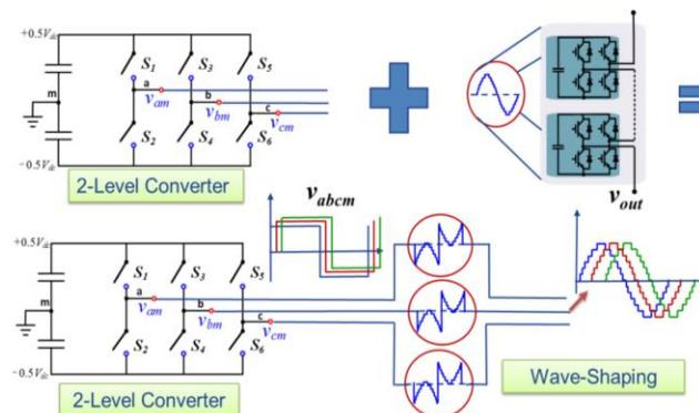
Figure: 4. Hybrid Voltage Source Multilevel Converter with Wave-shaping circuit on the AC side.
