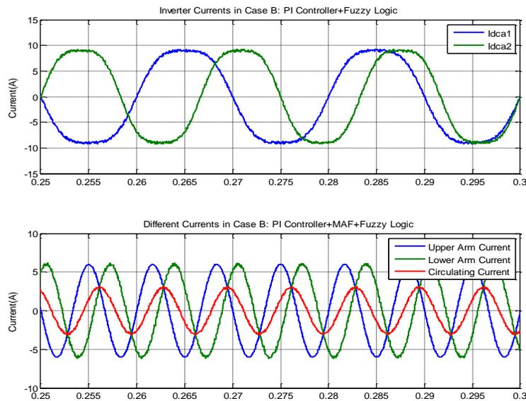
Figure: 9.2 Simulation Waveforms of Case B: PI Controller, Moving Average Filter with Proposed Fuzzy Logic controller.
