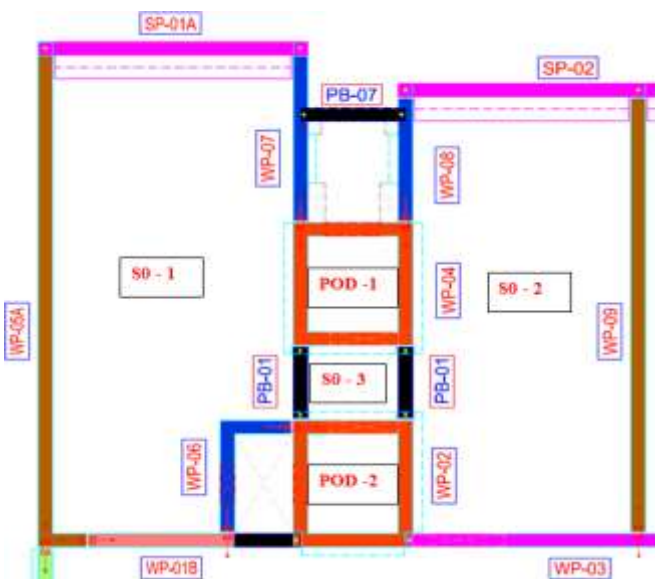
Fig.6 Pragati Towers-Precast Panel Layout for the Typical Apartment Floor Plan
