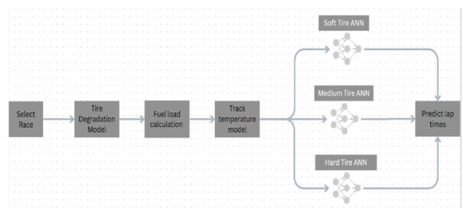
Fig- 1: System Architecture of our prediction model
