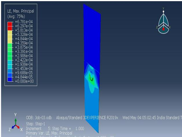
Linear strain for welded plate of nugget diameter 4.65 mm
