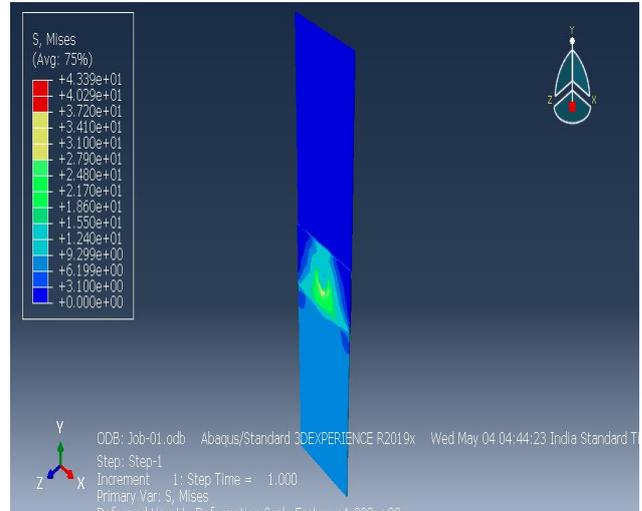
Vonmises stress for welded plate of nugget diameter 3.82 mm
