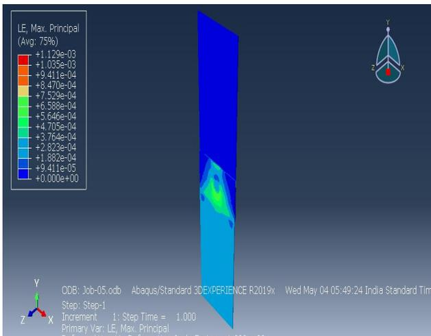
Linear strain for welded plate of nugget diameter 5 mm
