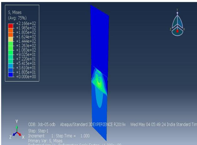
Vonmises stress for welded plate of nugget diameter 5 mm
