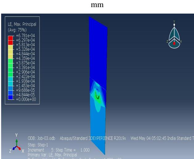
Linear strain for welded plate of nugget diameter 4.65 mm
