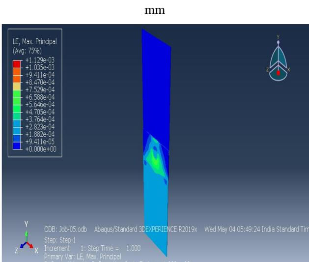
Linear strain for welded plate of nugget diameter 5 mm
