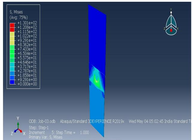
Vonmises stress for welded plate of nugget diameter 4.15 mm
