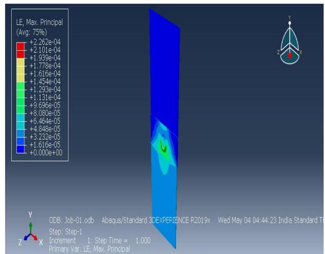
Linear strain for welded plate of nugget diameter 3.82 mm
