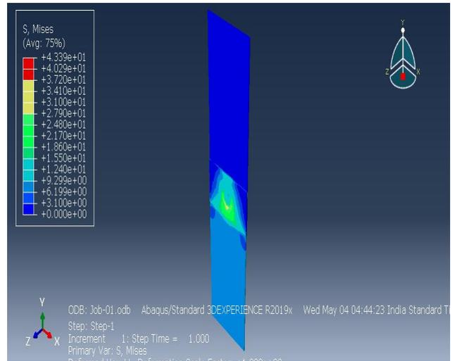
Vonmises stress for welded plate of nugget diameter 3.82 mm
