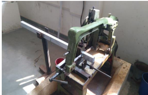
Fig -1: Cutting of Al6063
