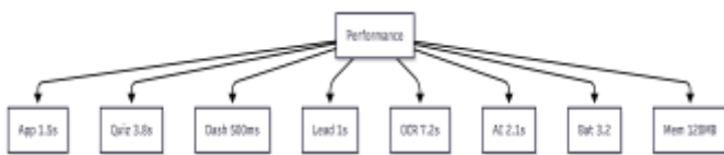
"Fig 8: PrepSprint Performance Metrics showing App Load Time (1.5s), Quiz Generation (3.8s), Dashboard Update (<500ms), Leaderboard Sync (<1s), and Battery Usage (3.2% per hour)—all meeting or exceeding targets."
