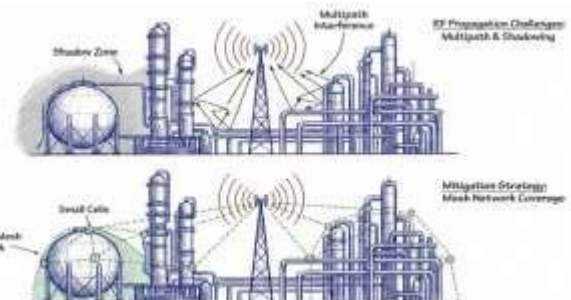
Figure 2: Mitigation strategy by using a "mesh" of small cells to fill coverage gaps.
