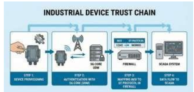
Figure 3: Onboarding and authentication of an industrial device on a private 5G network
