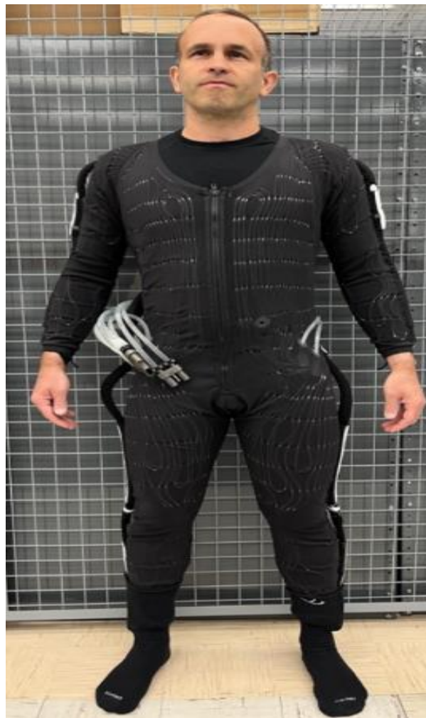
Figure 9: Liquid cooling and ventilation garment (St.Paul, et.al(2022))
