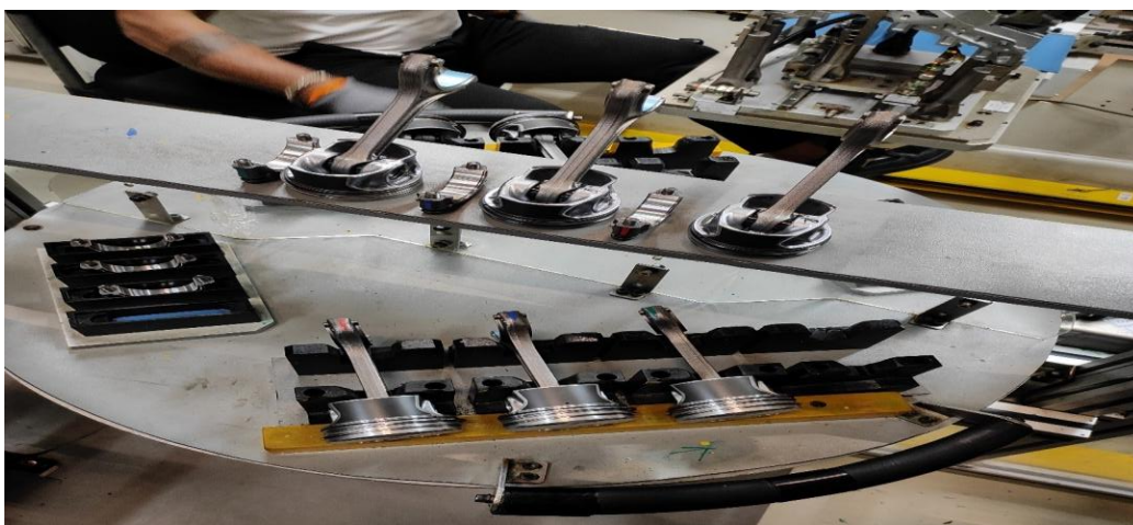
Pre Assembled Piston and Con Rod with Cap set Is Kept For Final assembly
