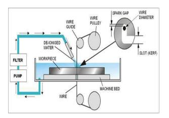
Fig 1.1: Schematic representation of EDM process
