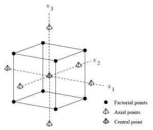
Fig 3.1: CCD showing 8 factorial points, 6 axial points and 6 center points used for experimentation.
