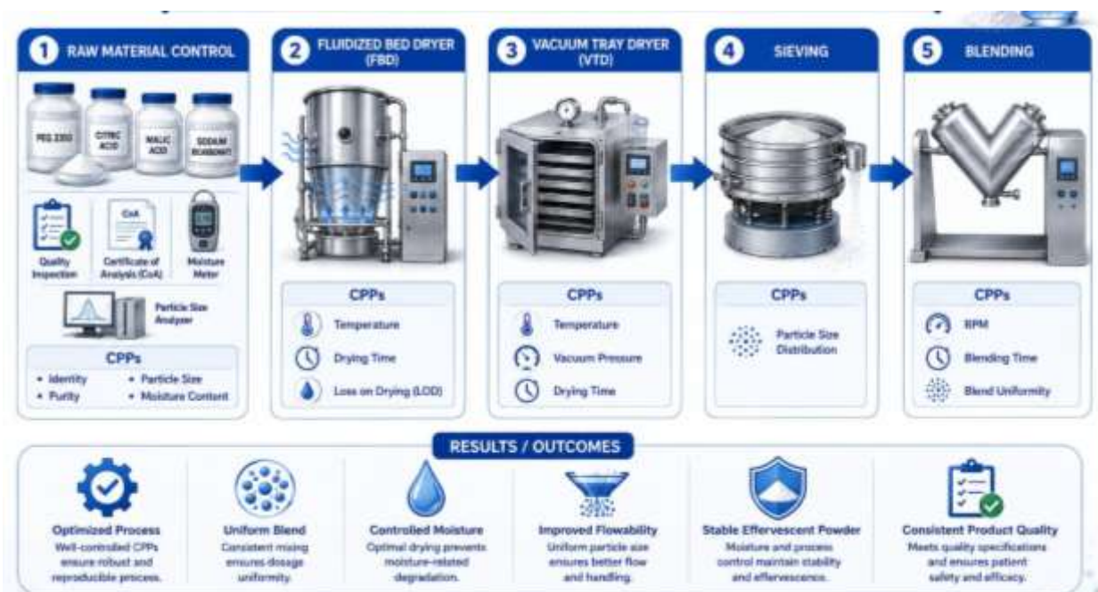
Figure 5 : Critical Process Parameters (CPPs) Flow Diagram
