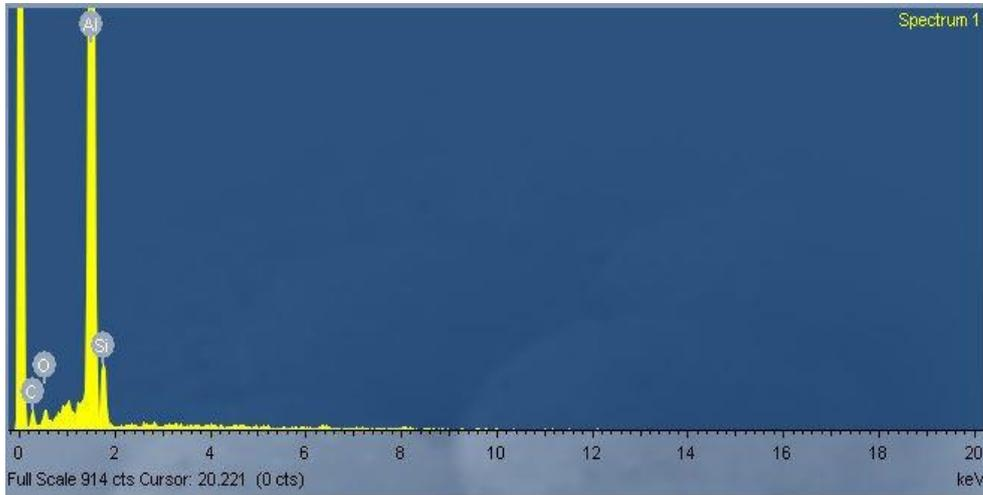
FIG 5.5(a) EDS microanalysis for as cast Al
