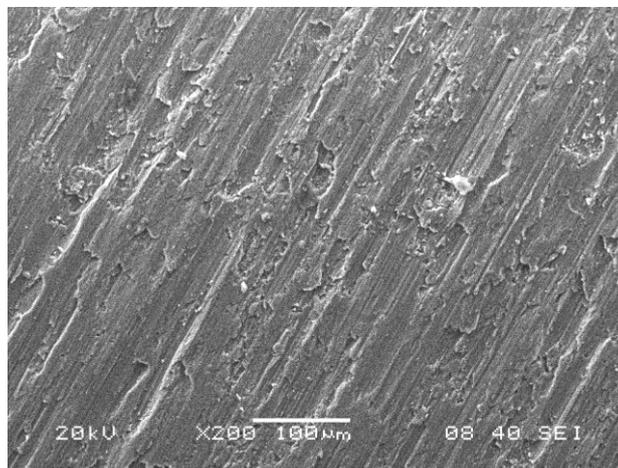
FIG 5.4 (b) SEM microstructure of Al-10% fly ash composite
