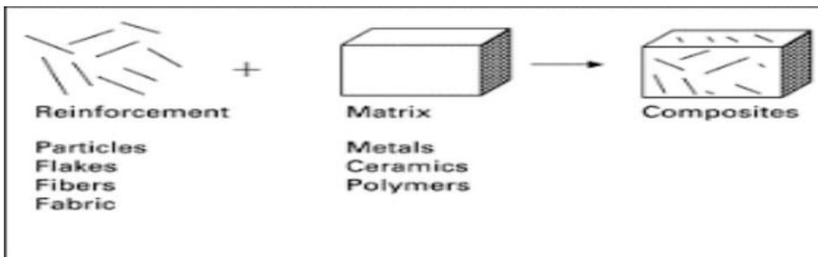
Fig 1: Schematic Diagram of Composite material
