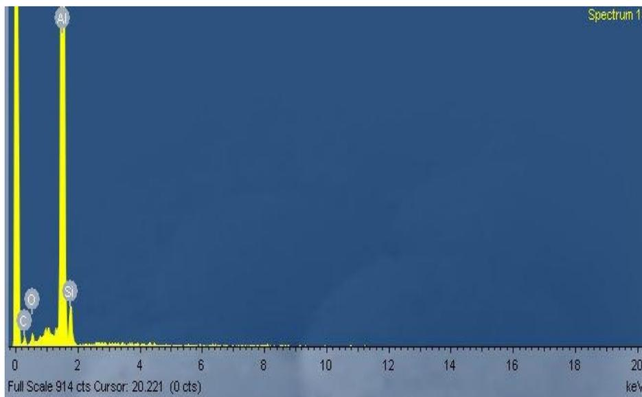
FIG 5.5(b) EDS microanalysis for Al-10% fly ash composite
