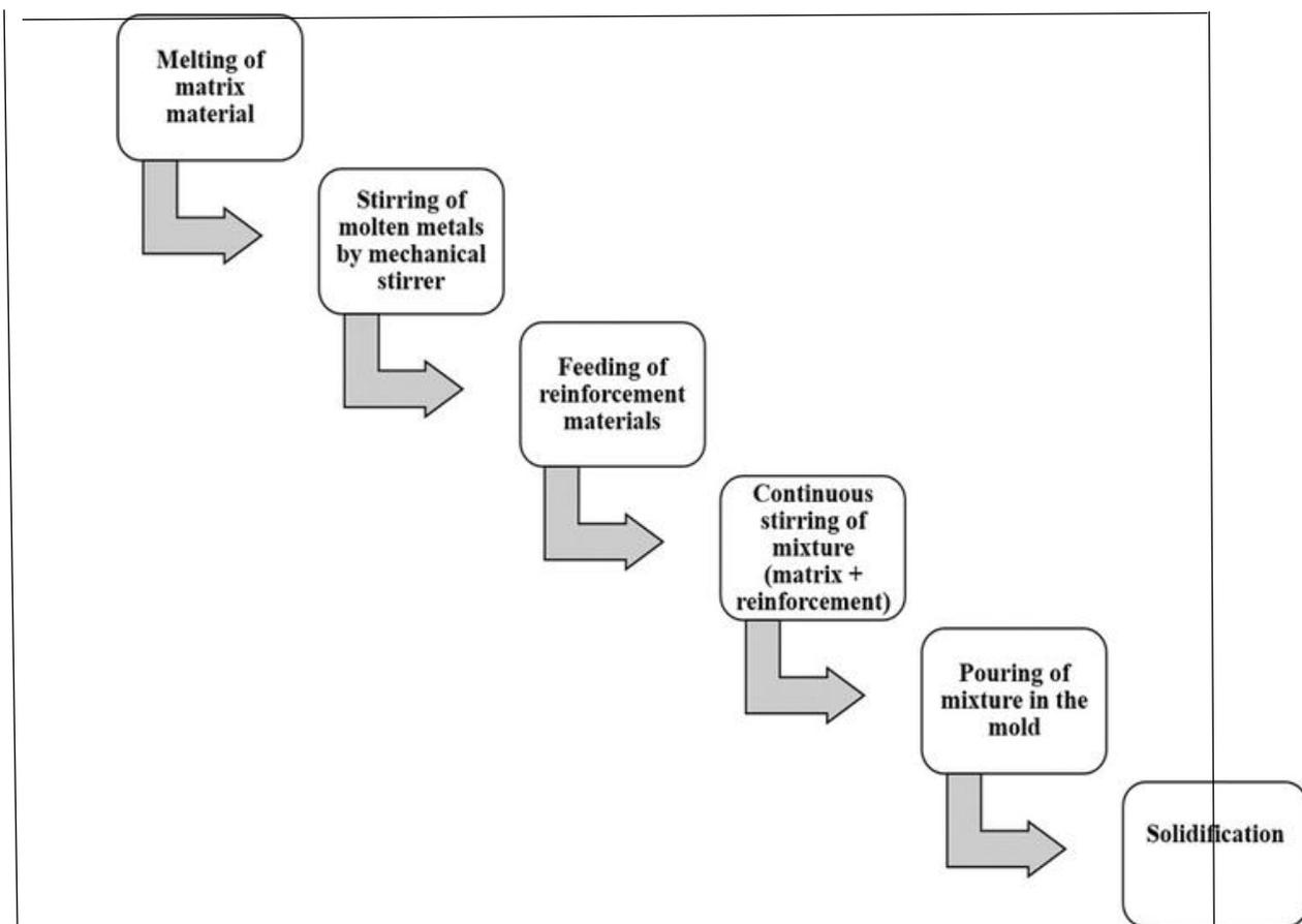
Fig: stir casting process
