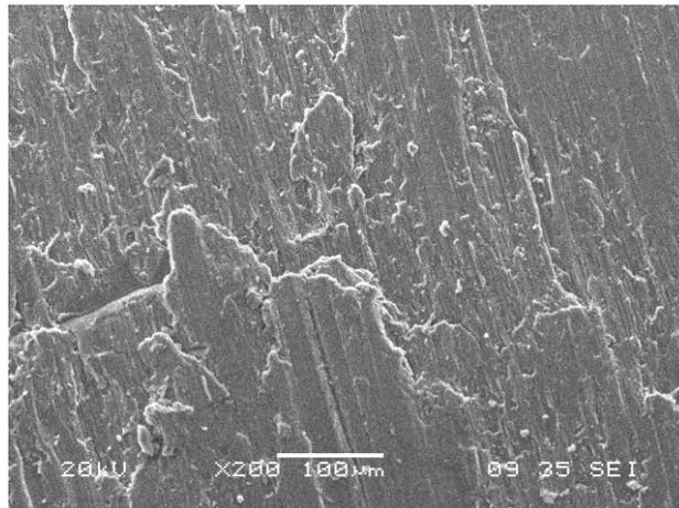
FIG 5.4 (a) SEM microstructure of as cast Al
