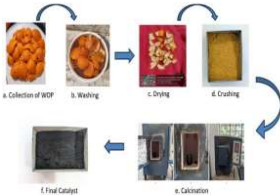
Fig -3. Preparation of waste orange peel catalyst using Muffle Furnace.
