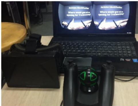
Figure 1: The set-up used- Oculus Rift, Razer Hydra and a laptop
