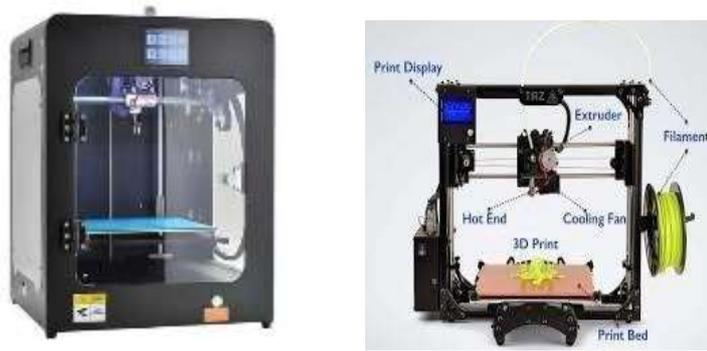
Fig: 4.1 Fused Deposition Modeling Machine
