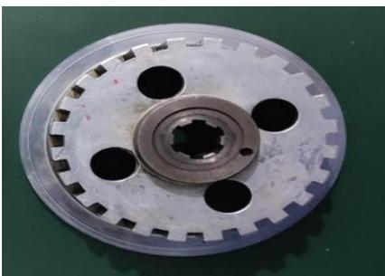
Figure 1. Two Wheeler Clutch Hub
