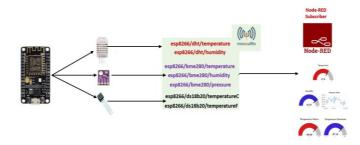
The ESP8266 board will be connected to the three types of sensors and data from the sensor will be published to the topics through the MQTT Broker. The Node red dashboard will subscribe to each of the topics to capture the published data and would be displaying it subsequently as it changes.
