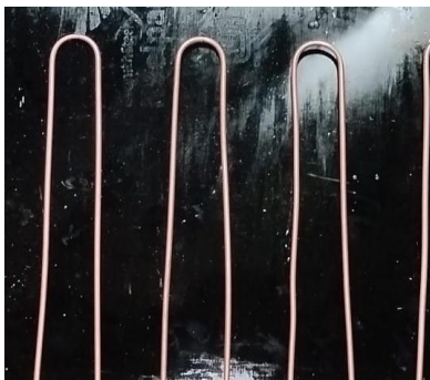
Figure 4 copper pipe bent for PHP line
