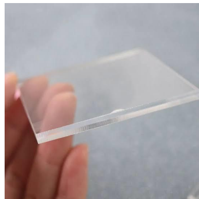
Figure 4 Replacement of glass with 6mm Acrylic Sheet
