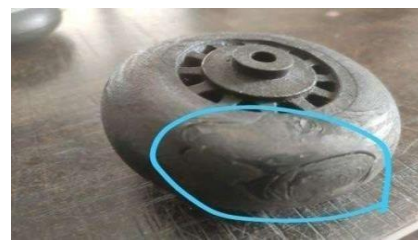
Figure 7.6 Flow Lines in Part
