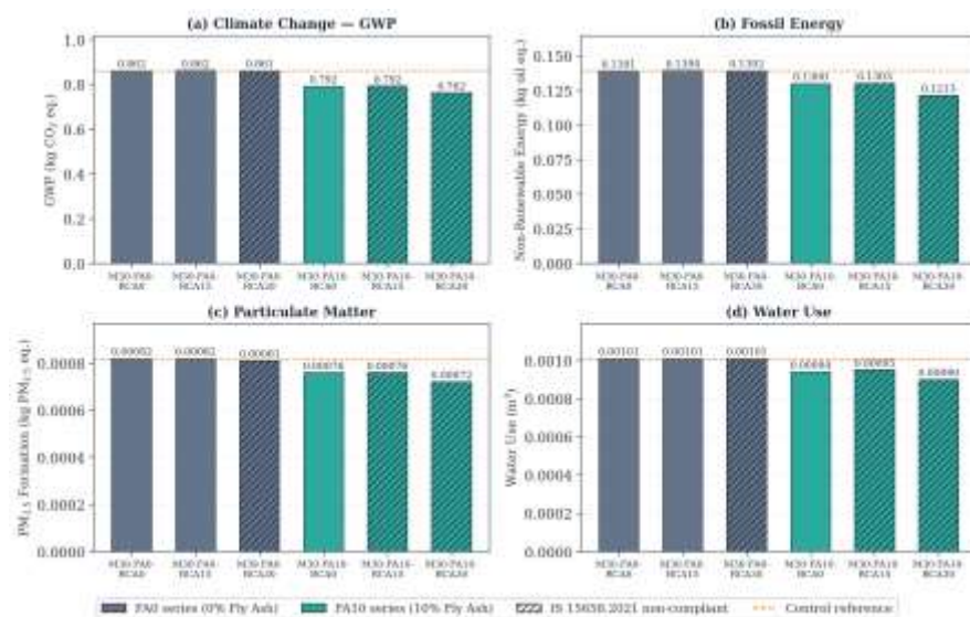
Fig. 3. Four-category environmental profile per paver block: (a) Climate Change, (b) Fossil Energy, (c) Particulate Matter, (d) Water Use.
