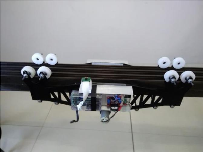
Fig. 3: Inspection robot on secondary track.
