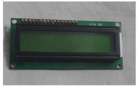
An LCD (Liquid Crystal Display) is a common output device used in fingerprint sensor-based attendance systems. It provides a visual interface for displaying information to users and administrators.
