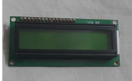
An LCD (Liquid Crystal Display) is a common output device used in fingerprint sensor-based attendance systems. It provides a visual interface for displaying information to users and administrators.
