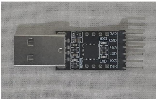
The CP2102 USB to TTL converter is a versatile and compact device commonly used for connecting various microcontroller and embedded systems to a computer or other USB-enabled devices. It can play a crucial role in a fingerprint sensor-based attendance system for configuring and interfacing the fingerprint sensor with the host system.
