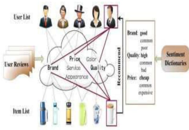
Fig. 2. The product features that user cares about are collected in the cloud including the words “Brand”, “Price”, and “Quality”, etc. By extracting user sentiment words from user reviews, we construct the sentiment dictionaries. And the last user is interested in those product features, so based on the user reviews and the sentiment dictionaries, the last item will be recommended.
