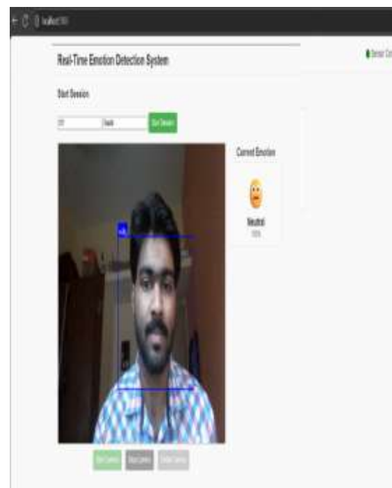
Figure 2. Real-time facial emotion recognition interface showing detection of the "Neutral" expression with 100% confidence. The system captures the user's face through a webcam, processes it using a CNN model, and displays the emotion and associated emoji instantly. A green indicator confirms sensor connectivity.
