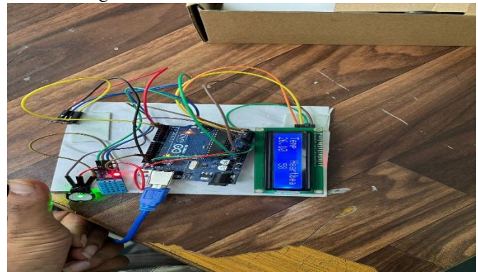
Fig.3.Complete hardware setup showing Arduino controller, sensors, keypad, and wiring connections.
