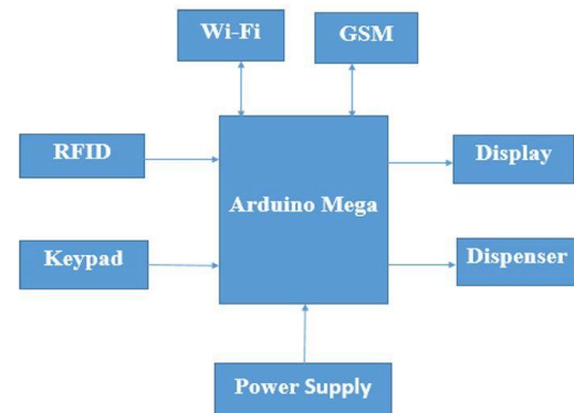
Fig. 1. Block diagram of the proposed virtual doctor system illustrating Arduino Mega as the central controller interfacing with RFID, keypad, display, dispensing unit, Wi-Fi, GSM, and power supply modules.
