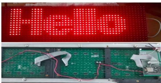
Fig: WEB BASED DISPLAY WITH WIFI CONNECTIVITY
