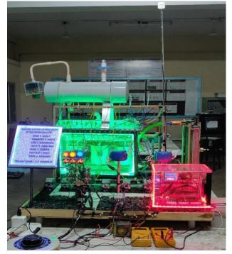
All the wiring connections from each equipment are brought forward up to the main supply point via fiber casing. As the main intentions were to have an oil-filled transformer for which the radiator with cooling fan setup is installed. The bottom surfacing is covered with gravels similar to the layout of a real substation. The setup also includes the main monitoring and protection kit and control panel for automatic
