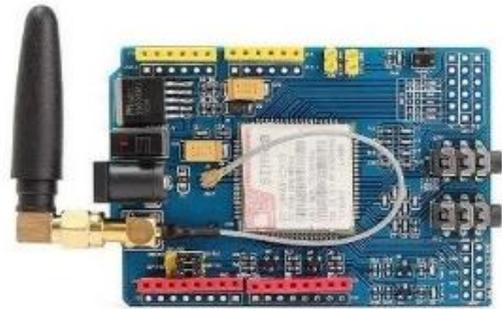
GSM is global system for mobile communication. GSM modem is device which is mobile phone having SIM card inserted for communication over wide range network. In this project GSM SIM 900 is used for smooth interface. Antenna is present on device
