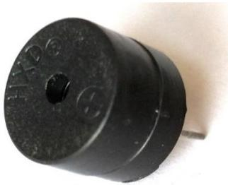
Buzzer is device used for audio signal. Buzzer has given DC voltage supply to convert into sound. The micro buzzer is used having positive terminal connected to supply and negative terminal to ground. The operating voltage is 4-8V DC and current is 30mA. It gives beep sound when relay is operated.
