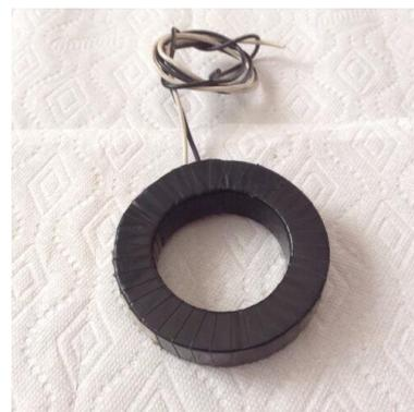
Current Transformer is used to sense the current present in the transformer. Current transformer converts high current of primary to low current of secondary winding which is proportional with primary winding. The ratio of CT used is 10/1mA.
