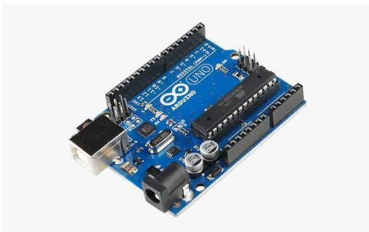
Arduino UNO is microcontroller based on ATmega328. It has 14 digital input/output pins and 6 analog pins. The operating voltage of Arduino is 5V. It is programmed with Arduino IDE which is Integrated Communication Area on USB type B and supplied with USB cable.
