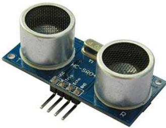
Ultrasonic sensor is used to measure distance of oil present in transformer tank by emitting ultrasonic sound waves. It has transmitter and receiver between which signal travels. In the project HC-SR04 model is used having 8mA operating current and supply given of 3.3V to 5V. The measuring angle is 15 degrees.
