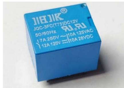
Relay is electrically operated switch which is used to control single or multiple circuits by only one signal. Relay has 3 contacts normally open, normally closed and common one. It turns to normally open or normally close from common after providing voltage to relay. The operating voltage of relay used in project is 12V consuming current of 150-200mA with trigger current 100mA.
