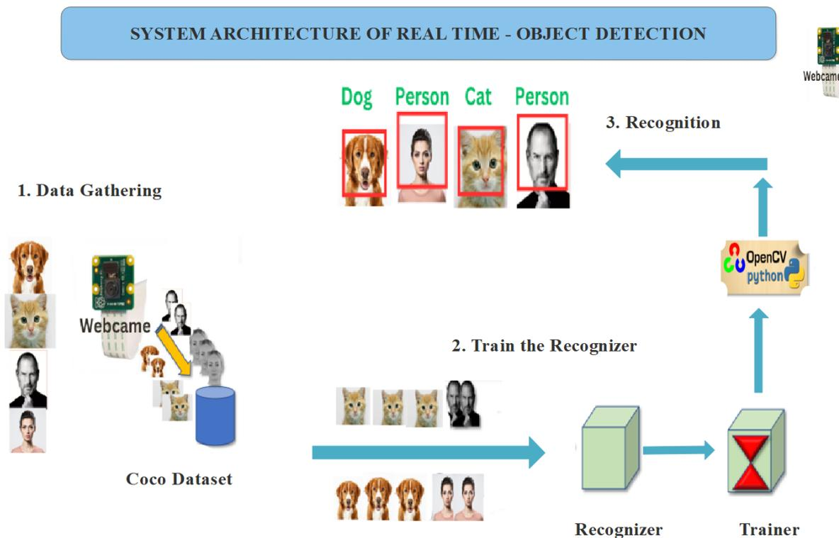
The system architecture involves a multi-stage process, beginning with data gathering through web cameras and the Common Objects in Context (COCO) dataset. Web cameras capture real-time visual data, while the COCO dataset provides a diverse set of labeled images for training the recognizer. The training phase employs a recognizer and trainer, utilizing advanced techniques such as convolutional neural networks
