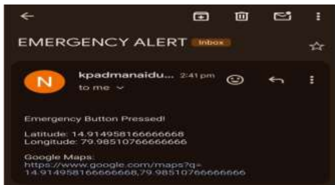
Fig 4: Emergency Alert Email Containing GPS Location
