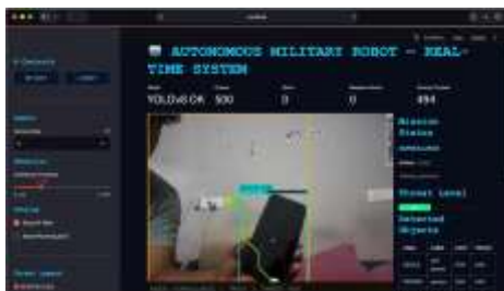
Fig. 3. System output: SURVEILLANCE mode — cell phone detected (conf=97%), A* path planned to target.
