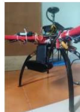
Figure 3: Baseline camera mount configuration showing rigid attachment to UAV frame
