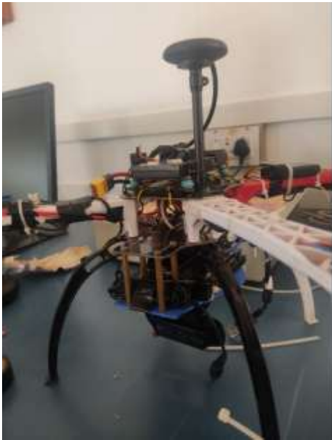
Figure 4: Angled front mount configuration with 45-degree downward camera orientation
