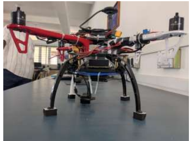
Figure 6: EPDM foam interface setup showing passive vibration damping layer
