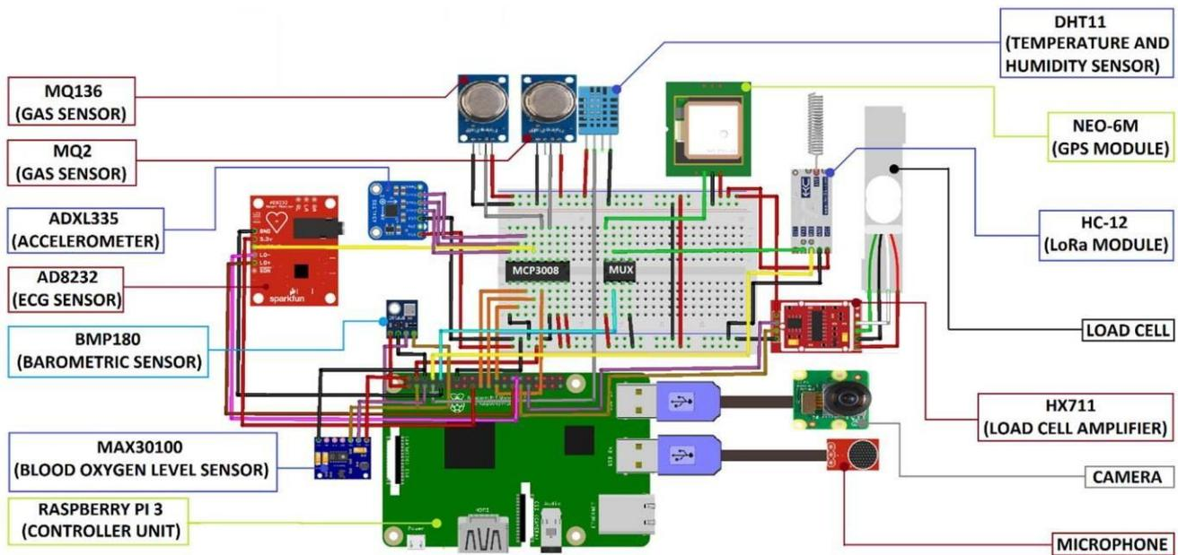
Fig.1. Circuit diagram of soldier's unit showing health and environmental sensors connected to Raspberry Pi controller
