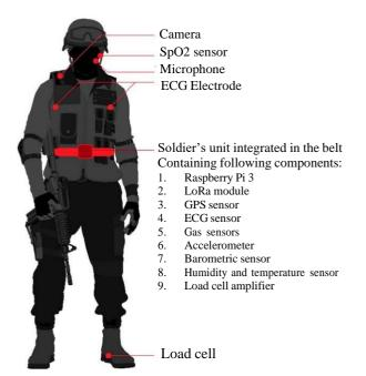
Fig. 2. Placement of WBASN (Wireless Body Area Sensor Network) on soldier's body
