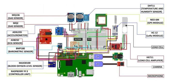
Fig.1. Circuit diagram of soldier's unit showing health and environmental sensors connected to Raspberry Pi controller
