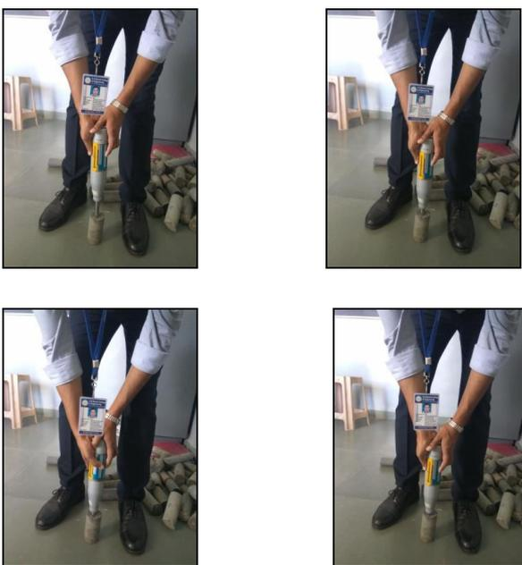
Figure 3: Performing Rebound Hammer Test on core samples.
