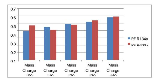
R600a refrigerants showed better performance for all mass charge of gas tested in this experiment except 110 gram as compared to R134a refrigerant. In the reading 140 gram of gas has highest COP & 100 gram of gas highest lowest COP.CW VS MASS CHARGE
