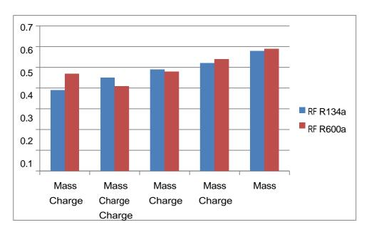
R600a refrigerants showed better performance for all mass charge of gas tested in this experiment except 110 gram as compared to R134a refrigerant. In the reading 140 gram of gas has highest COP & 100 gram of gas highest lowest COP.
